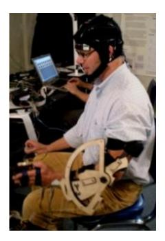
(PhysOrg.com) -- A portable, plugless, brain-to-computer interface using electroencephalography (EEG) electrodes strapped to the scalp has been developed by a team in the US. The device may allow paraplegics and others who have lost control of their limbs to control prosthetic devices and other equipment using their thoughts alone.
