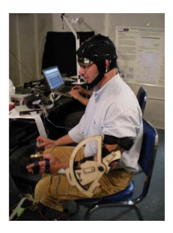
In tests at the University of Maryland, University of Michigan engineering researcher Brent Gillespie uses a prototype of a device that provides feedback to the wearer's arm while objects are moved with a prosthetic 'hand,' a gripper. The prototype, which incorporates noninvasive monitoring of electrical activity and blood-oxygen levels in the brain, may be incorporated into next-generation prosthetic arms. Credit: J. Contreras-Vidal/University of Maryland
