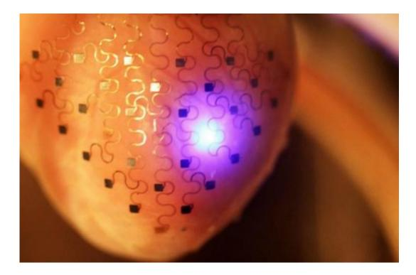
The "heart sock" is made of a thin silicone membrane embedded with flexible sensors that can monitor vital signs.
