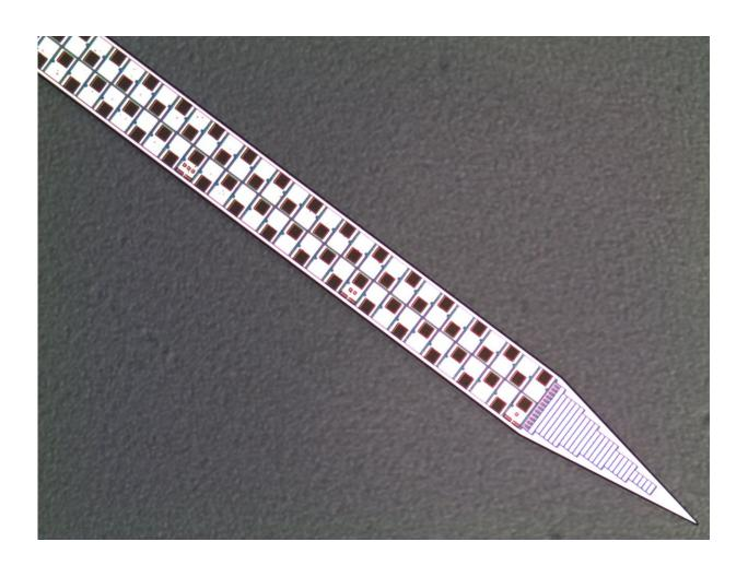
The Neuropixels probe places hundreds of recording electrodes across a large span of a rodent's brain, so that researchers can collect more meaningful data in a single experiment than other technologies currently allow. Credit: Timothy Harris Lab, Janelia Research Campus
