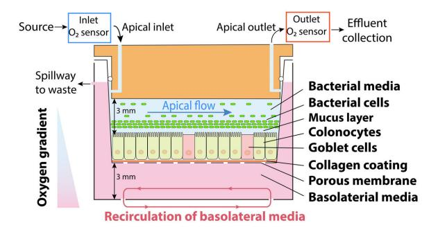
This schematic shows a novel device that MIT engineers have built, allowing them to grow human colon tissue along with oxygen-intolerant bacteria that normally live in the human digestive tract. Credit: Jianbo Zhang
