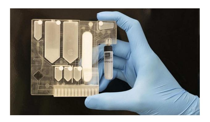
GeneCapture's unique disposable cartridge design enables rapid multi-pathogen identification directly from samples. Credit: GeneCapture
