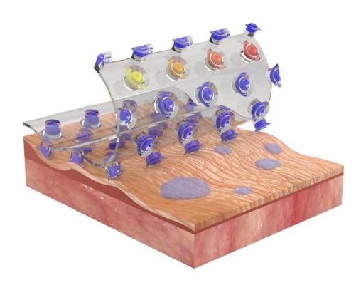
Schematic illustration of the adhesive patch with diving beetle-inspired suction
