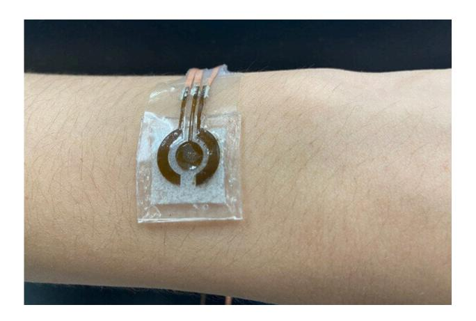
Penn State researchers developed a prototype of a wearable, noninvasive glucose sensor, shown here on the arm. Credit: Jia Zhu
