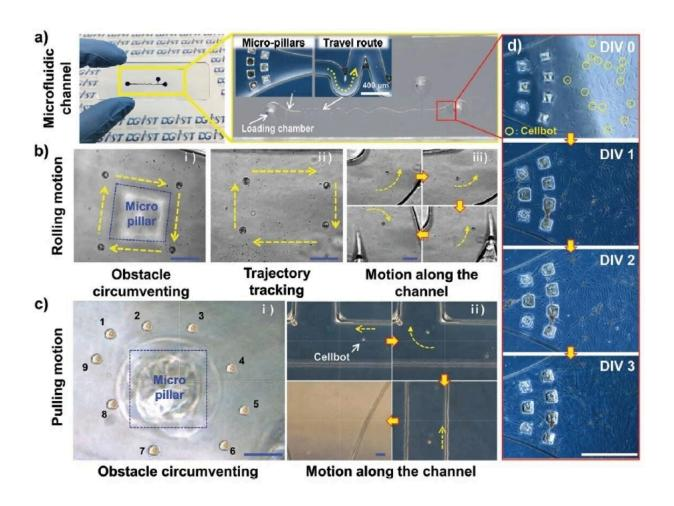
In vitro magnetic actuation of the Cellbots in a microfluidic channel. a) Fabricated microfluidic channel with loading chamber, micro-pillars, and tortuous route. b) Rolling motion of the Cellbots under a rotating magnetic field (scale bar =  $50 \mu m$ ). c) Magnetic pulling motion of the Cellbots under a magnetic field gradient (scale bar =  $50 \mu m$ ). d) Co-cultivation of the Cellbots with 2D attached hNTSCs in the microfluidic channel (scale bar =  $500 \mu m$ ). DIV, days in
