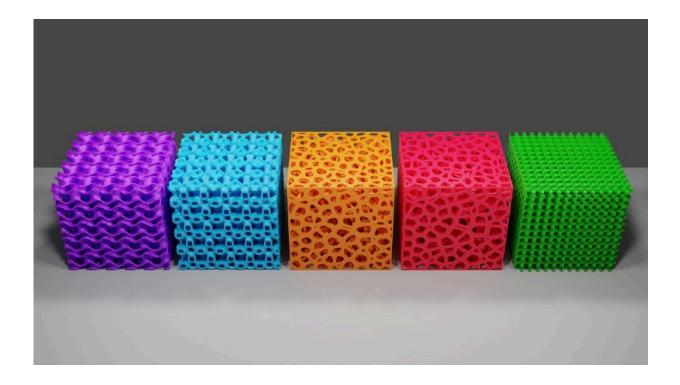
Different designs used in the study, comprising 2 TPMS-type structures (1st and 2st from the left), 2 Trabecular-like structures (3rd and 4th from the left), and the typical Lattice currently used as a control (far right). Credit: Loughborough University
