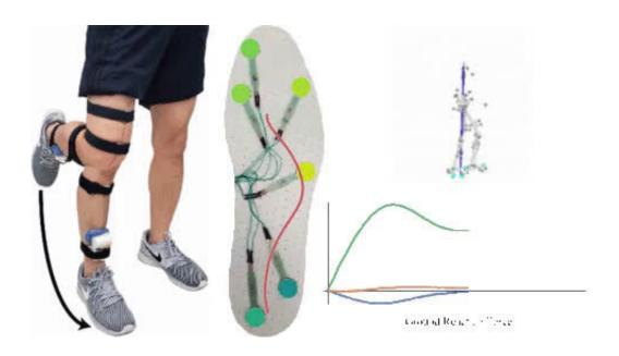
An interdisciplinary team of University of Massachusetts Amherst researchers has developed a low-cost shoe insole, equipped with force-sensitive resistors (FSR), that aims to improve the management of health conditions that impair mobility, such as stroke, Parkinson's disease and osteoarthritis.
