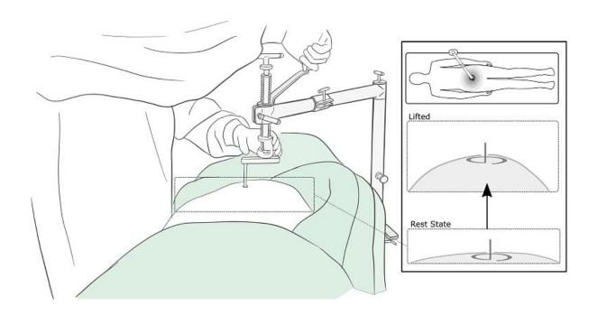
A diagram showing how the RAIS retractor is used to lift the abdominal wall during surgery. Credit: University of Leeds/Dr Pete Culmer
