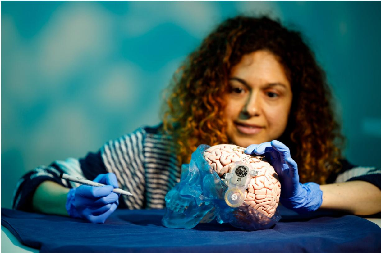
ABILITY is a fully implantable neural recording system designed to amplify and wirelessly transmit high channel count, high frequency neural data from the brain to a computer in order to restore communication and independence for people with severe paralysis. Credit: Wyss Center
