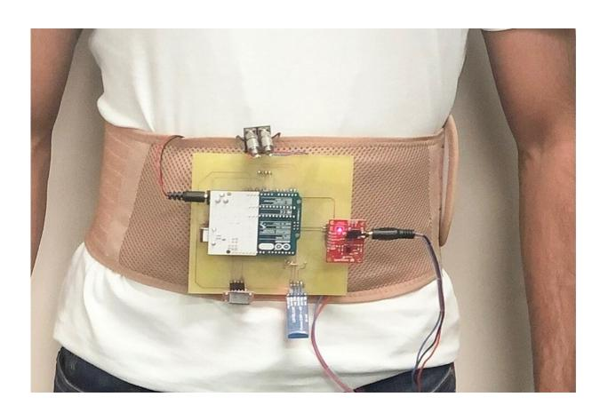
The lightweight belt continuously monitors all of the physiological parameters associated with heart failure in real time, 24/7. Credit: FAU College of Engineering and Computer Science
