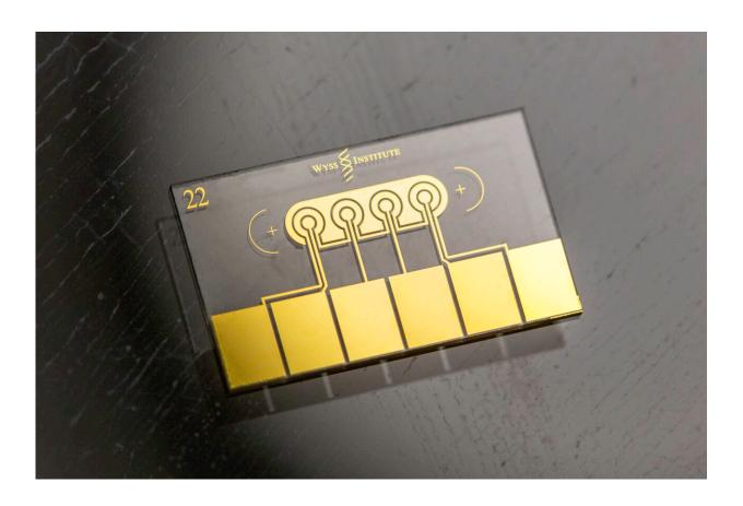
The Wyss Institute's eRapid electrochemical sensor platform enables the multiplexed, fast, and inexpensive detection of biomarker molecules specific for infectious and other diseases at the point-of-care. Credit: Wyss Institute at Harvard University
