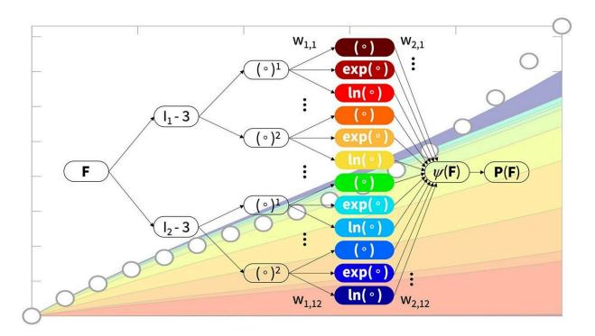
Out of 4095 possible models, the network autonomously discovers the model and parameters that best explain the stresses in human brain tissue. Credit: Ellen Kuhl
