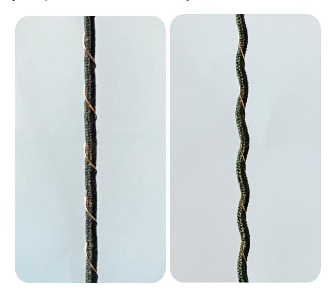
Garn: A rigid wire (orange) is wrapped in spirals around a length of elastic rubber (black)—both are conductive. Left slack, right stretched. Credit: Tyler Cuthbert / ETH Zurich
