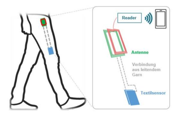
The textile sensor and antenna form an electrical circuit. When the sensor stretches, the antenna sends a signal that can be read by a smartphone. Credit: Valeria Galli / ETH Zurich
