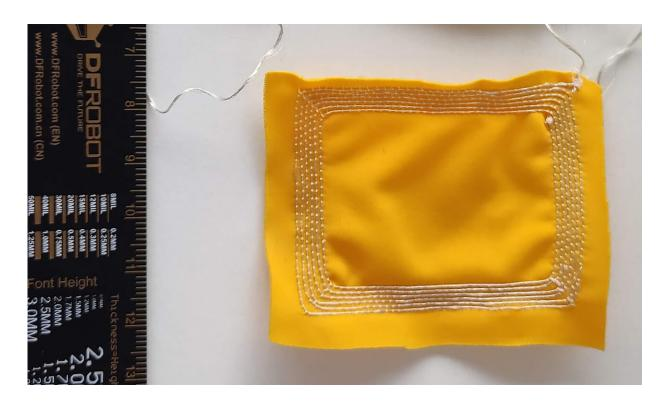
The antenna is sewn directly onto the material in loops. Credit: Valeria Galli / ETH Zurich
