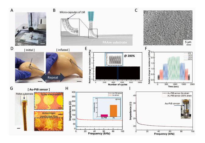
(A) The photograph of meniscus-guided coating of EGaIn\* (EGaIn liquid metal particle) on a PAAm substrate. Scale bar, 10 mm; (B) Schematic illustration of printed EGaIn\* on PAAm substrate; (C) SEM images of printed EGaIn\* on PAAm substrate; (D) Photograph of mimicking micturition using artificial bladder. Scale bar, 5 mm; (E) The plot of relative resistance change of the strain sensor under repeated 10,000 cycles at 200% strain; (F) Plot of relative
