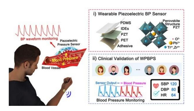
Schematic illustration of the overall concept for a wearable piezoelectric blood pressure sensor (WPBPS). Credit: The Korea Advanced Institute of Science and Technology (KAIST)
