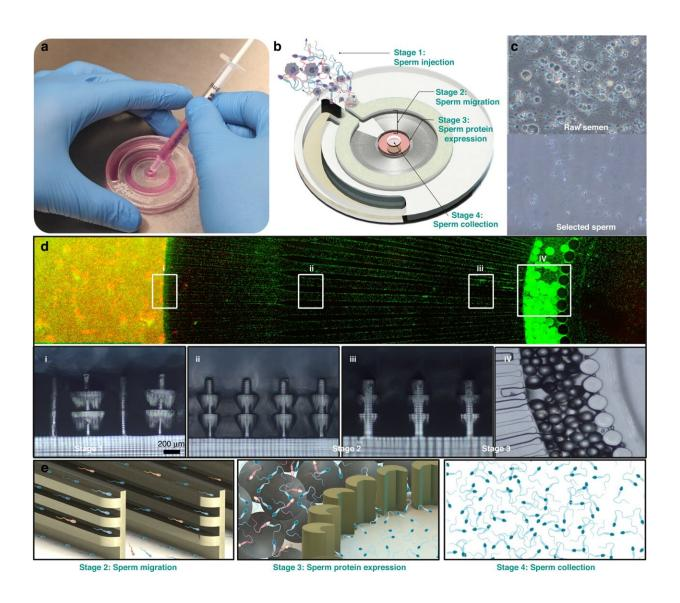
Overview of the sperm selection process within the microfluidic device and representative geometry. a Image of the device filled with food dye for visualization. b Schematic overview of the device showing each stage of
