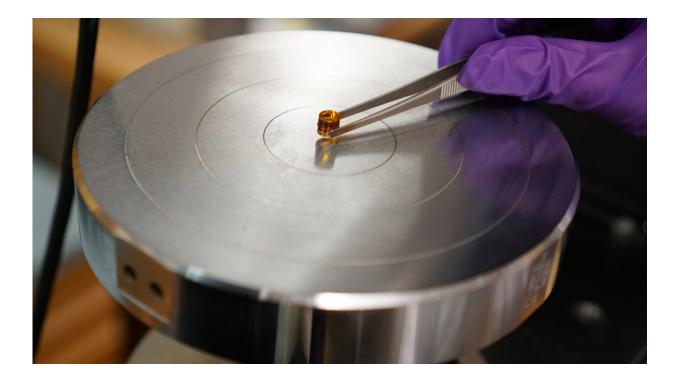
Placing the hydrogel on a compression machine. Credit: Alex Walls
