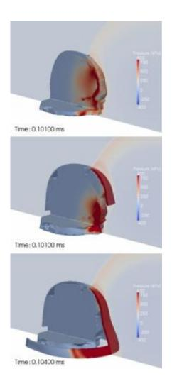
These images show the pressure waves that are transmitted to the brain tissue for the three simulation scenarios considered by Radovitzsky's team: unprotected head (top), head with helmet (middle), and head with helmet and face shield (bottom). The face shield clearly prevents the direct transmission of blast energy into the brain. Images: Michelle Nyein
