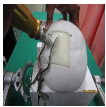
A perforator creates a bur hole in the model of a skull. The model, produced using the latest generation of multimaterial 3D printers, is composed of a variety of materials that simulate the various consistencies and densities of human tissues encountered during neurosurgery. Credit: © American Association of Neurosurgeons, 2013.
