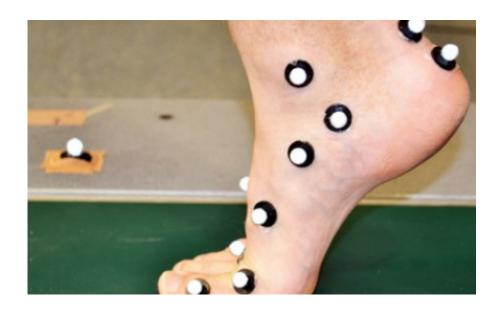
Retro-reflective skin markers for three-dimensional motion capture were applied to the right foot of each human participant of a UQ-led study on how foot muscles support the arch.
