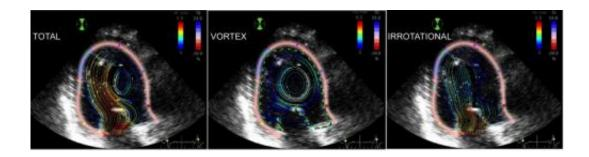
Researchers separeted the total 2D-velocity field of intra-ventricular flow (left) into a vortex field (center) and an irrotational field (right). Credit: Jacobs School of Engineering
