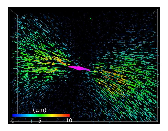
The above image shows the measurement of single-cell traction force using gel deformation and a fibrous nonlinear elastic model. Each arrow represents the discrete displacement of a fluorescent bead bonded to a collagen fiber. Credit: Matthew Hall/Provided
