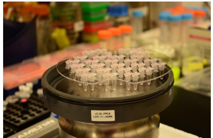
The sonicator used for Protein Misfolding Cyclic Amplification (PMCA), the amplification technique used to detect abnormal prion proteins in patient blood. Credit: Luis Concha-Marambio
