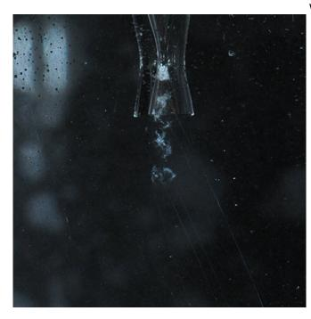
The researchers used a certain type of nozzle to create the cavitation bubbles which removed the plaque when they collapsed. Credit: Hitoshi Soyama
