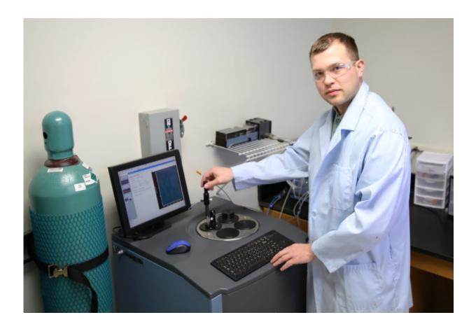
Andrey Zakharchenko, a doctoral candidate in the UGA Nanostructured Materials Lab within the College of Family and Consumer Sciences, uses a micro calorimeter to monitor the release of drug molecules from nanoparticle carriers. Credit: Cal Powell
