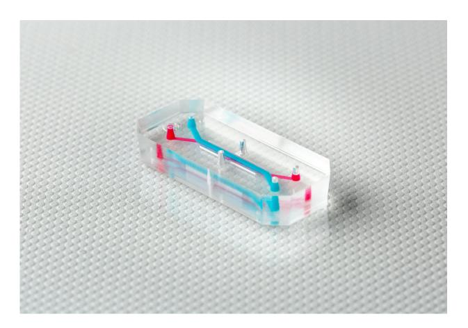
Microengineered Organ-Chip is made out of a flexible polymer that features tiny channels that can be lined with thousands of living human cells. Credit: Emulate, Inc.
