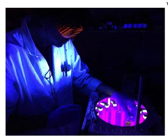
Charitha Guruge, a Ph.D. student at Florida Institute of Technology, places a sample of an inactive, or "caged," version of the neurotransmitter glutamate in a photo reactor. The UV lamps in the reactor activate the neurotransmitter, which is a key tool for neuroscientists to use in mapping the enormously complex brain circuitry. Credit: Florida Institute of Technology
