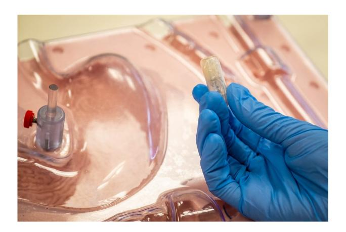
Measuring about 3cm by 1cm, the EndoPil prototype capsule contains a balloon that can be self-inflated with a handheld magnet once it is in the stomach, thus inducing a sense of fullness. Its magnetically-activated inflation mechanism causes a reaction between a harmless acid and a salt stored in the capsule, which produces carbon dioxide to fill up the balloon. Credit: Nanyang Technological University
