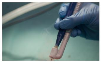
Flue gas created by an electric knife is fed directly into the measurement system. Credit: Antti Roine
