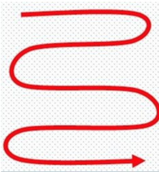
The S-shaped pattern for cleaning a surface without recontaminating parts of it. Credit: Brett Mitchell, Author provided
