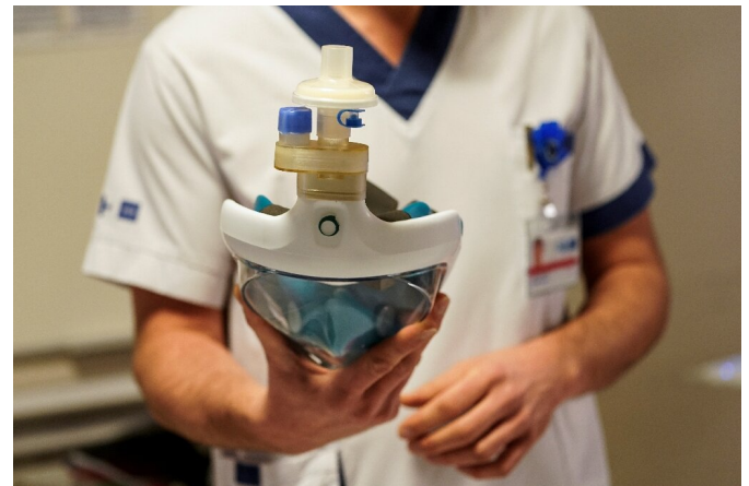
A medical worker tests a Decathlon snorkeling mask, with a 3D-printed respiratory valve fitting attached, at the Erasme Hospital in Brussels
