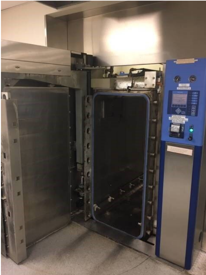
The researchers used an autoclave, which was one of four sterilization methods they tested on the masks. Credit: University of Manitoba
