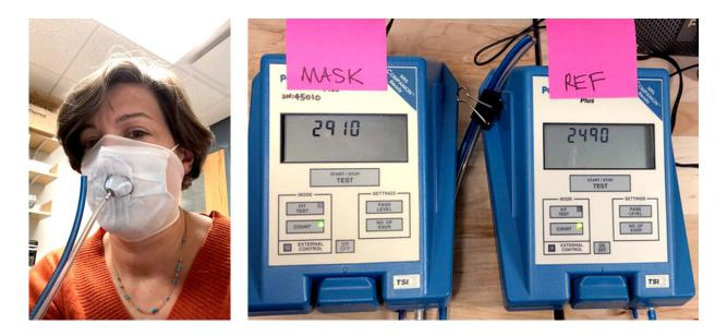
Fernandez, who tested 10 different types of homemade masks made with different materials, used nylon stocking layers to make for a tighter fit. The optimized fit improved the performance of all face masks—homemade or not. Credit: Loretta Fernandez
