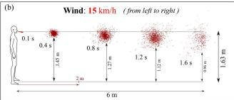
Saliva droplets can travel large distances, depending on environmental conditions such as wind speed, temperature, pressure and humidity. Wind shown blowing left to right at speeds of 4 kph (top) and 15 kph (bottom) can transport saliva droplets up to 6 meters (18 feet). Credit: the authors
