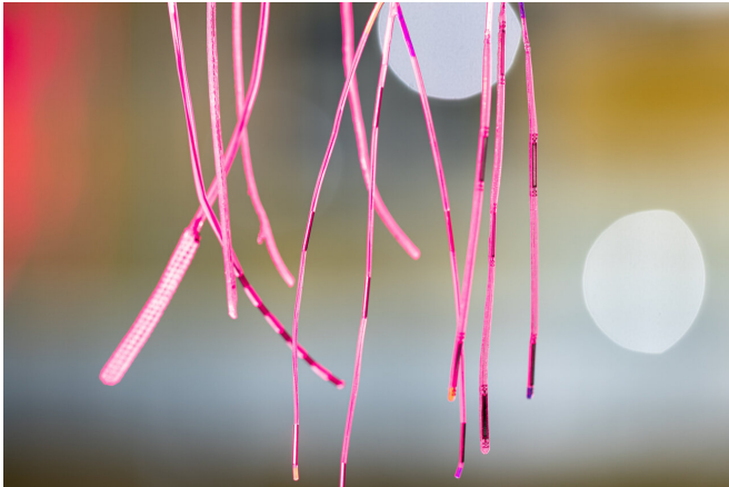
Subscalp electroencephalography (EEG) systems include sensors that measure brain activity from beneath the scalp for long periods of time. Credit: Wyss Center
