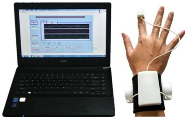
ISWD for the quantification of Parkinsonian tremors and bradykinesia. Credit: Prof. Dai's group
