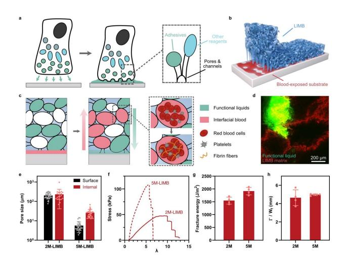
Design of LIMB. a) Schematic illustration of marine organisms that contain interconnected micropores for adhesiveness and transport of liquid reagents. b) Schematic of LIMB adhering on blood-exposed substrates. c) Schematics showing that LIMB can uptake interfacial fluid, secrete functional liquids, and coagulate blood, thereby providing adhesion, hemostatic, and sealing function. d) Confocal image of rhodamine-labeled LIMB (red) containing micropores,
